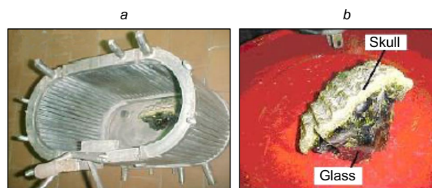
Figure 4. View of a cold crucible melter with a piece of glass manufactured in it (a) and a view of this piece with the protective layer made of glass batch material (skull) which separates the glass melt inside the cold crucible melter from its water-cooled tubes (b). 36
