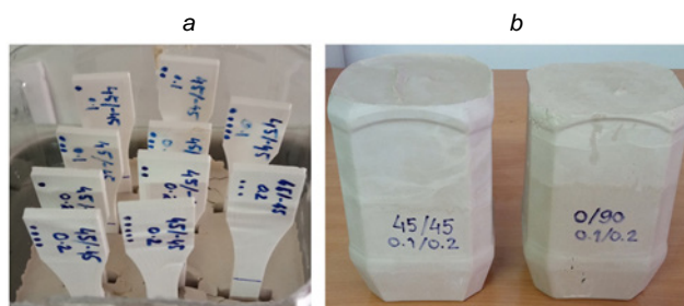
Figure 10. Example of heat post-treatment in gypsum: (a) parts partially immersed in gypsum; (b) pre-annealing forms with parts fully immersed in gypsum. 88 The figure is published under a Creative Commons Open Access license.
