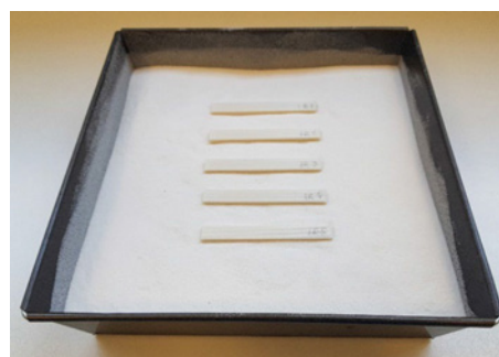
Figure 8. Specimens in container filled with \text{Al}_2\text{O}_3 powder. 105 Figure published under the Creative Commons CC BY open access license.
