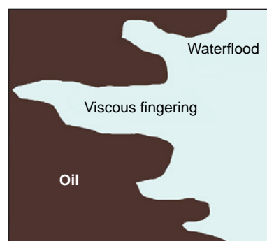
Figure 3. Viscous fingering effect upon water flooding of an oil formation.
