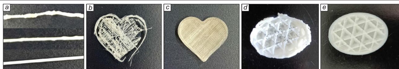
Figure 4. (a) Filaments produced by the extrusion at 200°C using PE (homopolymer, Ni46 /MgO catalyst, upper image) and copolymers with 0.5 mol.% C018 ( Ni46 /MgO catalyst + Ni48 /MgO, middle image; and Ni46 + Ni48 /MgO, lower image). 3D Printed samples made of (b) LLDPE, (c) copolymer with 1.1 mol.% C018 , and composites (3 : 7 by weight) based on (d) PLA/HDPE and (e) PLA/copolymer with 1.1 mol.% C018 [PLA is poly( L -lactide), HDPE is linear high-density polyethylene]. 148 Reproduced with permission from Nature (CC-BY).
