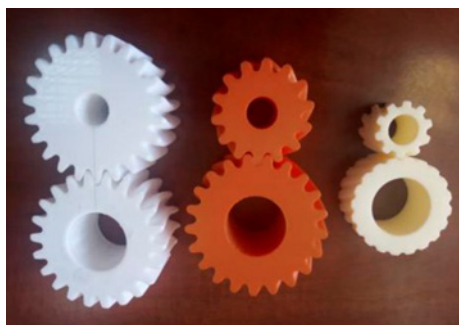
Figure 29. 3D-printed gears with different types of meshing. 193 ©International Journal of Mechanical Engineering and Robotics Research, 2020.
