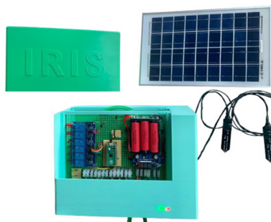
Figure 49. Solar-powered irrigation system. 278 ©IOP Publishing, 2022.
