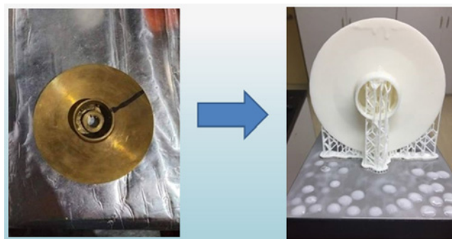
Figure 27. Metal impeller of a solar-powered pump and its plastic counterpart made using 3D printing. 188 © De Gruyter, 2021.
