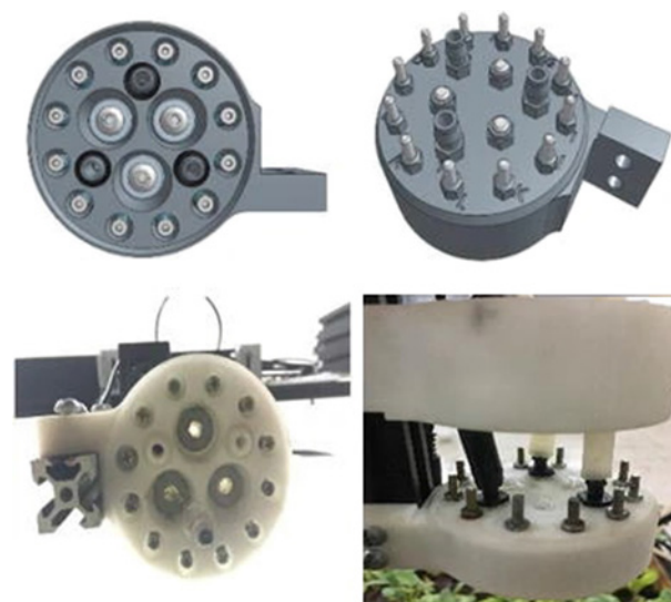
Figure 43. 3D model and photo of the prototype magnetic clutch for FarmBot in two projections. 242 © Springer Nature, 2018.
