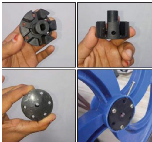
Figure 26. 3D-printed ABS wheel hub and wheel assembly. 187 © AIP Publishing, 2021.
