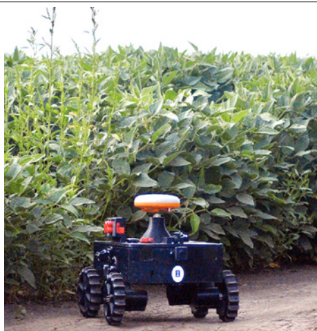
Figure 36. Agricultural robot assembled using 3D-printed parts and equipped with a navigation system and computer vision algorithms for automatic counting of corn stalks and other phenotyping tasks. 217 © Springer Nature, 2018.
