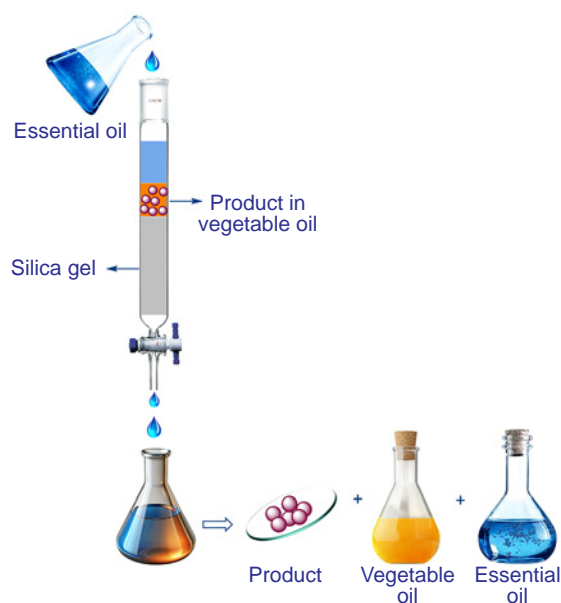
Figure 11. Scheme of the target product isolation using preparative column chromatography.
